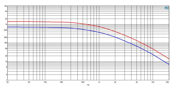
Figure 11: Damping factor vs. frequency  $4\Omega$  (blue) and  $8\Omega$  (red)
