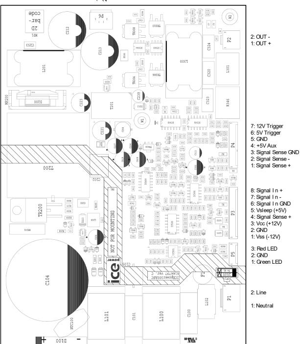
Figure 2: ICEpower300AS1 connections
