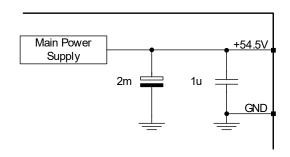
Figure 16: VD (+54.5V) output
