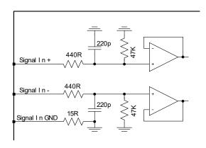
Figure 14: Balanced input buffer
