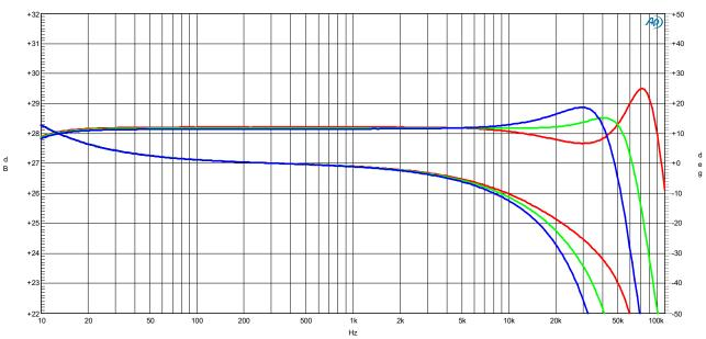
Figure 3: Frequency response in 4 $\Omega$  (blue), 8 $\Omega$  (green) and open load (red). Top – amplitude. Bottom – phase
