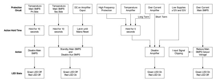
Figure 27: Block diagram of protection features.
