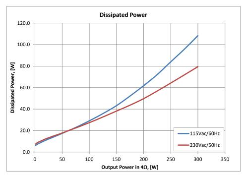
Figure 13: Dissipated power vs. output power
