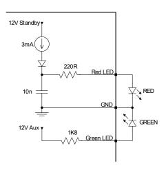
Figure 18: LED indication for St-by/ON
