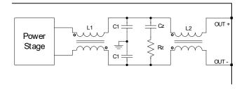
Figure 15: Output filter section with compensating Zobel network
