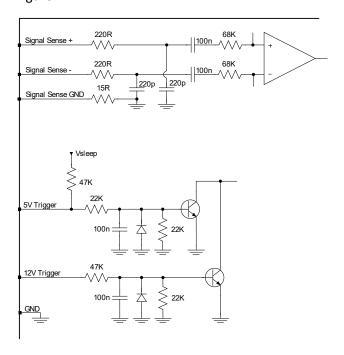
Figure 17: Signal Sense and Trigger inputs
