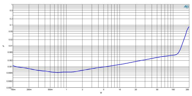
Figure 8: CCIF IMD vs. Output Power,  $R_L = 4\Omega$ ,  $f_1 = 18$ kHz,  $f_2 = 19$ kHz. 1kHz
