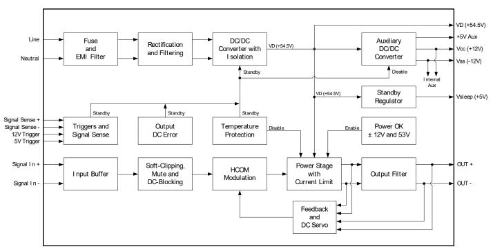
Figure 1: ICEpower300AS1 block diagram
