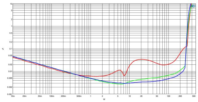
Figure 4: THD+N vs. Po at 100Hz (blue), 1kHz (green) and 6.67kHz (red),  $4\Omega$ , 230Vac/50Hz
