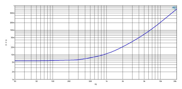
Figure 10: Output impedance at the output terminals
