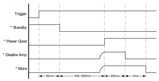
Figure 23: Power up from trigger high. \* denotes an internal signal
