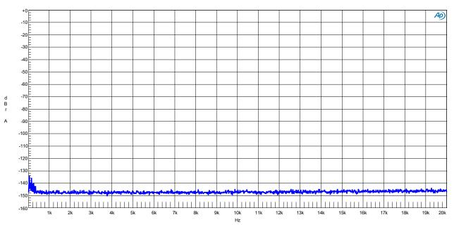
Figure 6: Idle noise (16K FFT). Residual =  $75\mu V(A)$
