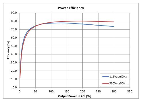
Figure 12: Efficiency vs. output power
