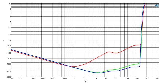
Figure 5: THD+N vs. Po at 100Hz (blue), 1kHz (green) and 6.67kHz (red),  $8\Omega$ , 230Vac/50Hz
