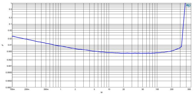
Figure 9: TIM vs. output power. R  $_{\! L}$  =  $4\Omega$
