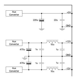
Figure 19: +5V and ±12V Auxiliary
