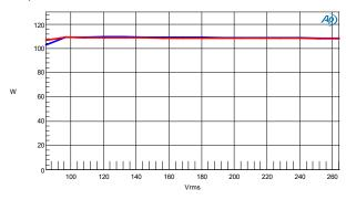
Figure 13: Output power per channel vs mains, 50Hz (blue), 60Hz (red)
