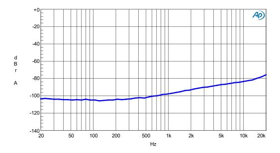
Figure 9: Typical channel separation 20-20kHz, 0 dB @ Po = 12.5 W / 4  $\Omega$
