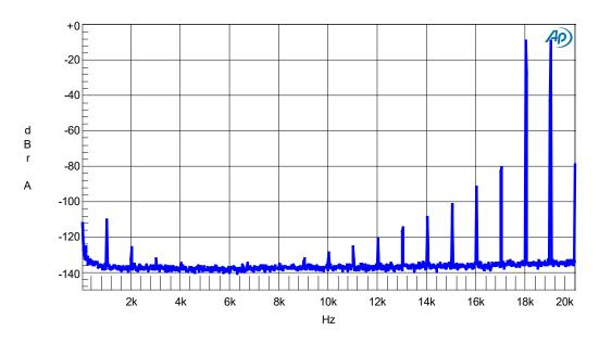
Figure 8: Intermodulation (16kFFT) 0-20kHz @ 0dB = 100 W/4  $\Omega$
