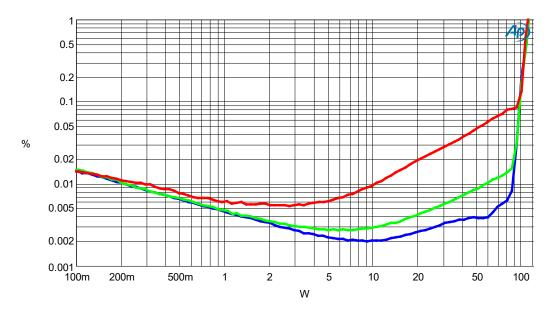
Figure 5: THD+N vs power @ 100 Hz (blue), 1kHz (green), 6.66kHz (red),  $R_L$  = 4  $\Omega$
