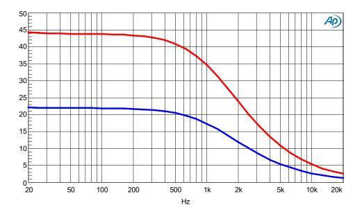
Figure 11: Damping factor vs frequency 20-20kHz,  $4\Omega$  (blue),  $8\Omega$  (red)
