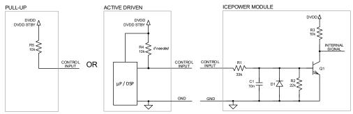
Figure 25: Control input interface schematics
