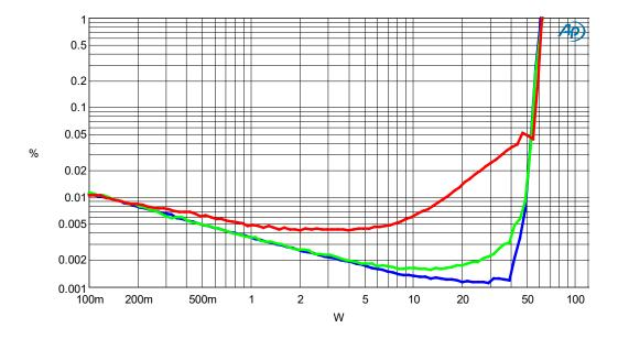
Figure 6: THD+N vs power @ 100 Hz (blue), 1kHz (green), 6.66kHz (red), R $_{\rm L}$  = 8  $\Omega$
