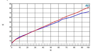
Figure 17: Dissipated power vs. output power per channel, 230V/50Hz (blue), 115V/60Hz (red)
