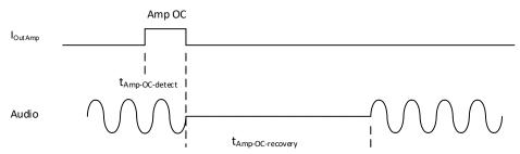
Figure 21: Speaker output overcurrent timing
