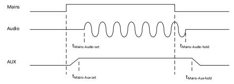
Figure 18: Power up timing
