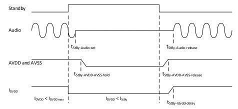
Figure 19: Standby timing on auxiliary supplies
