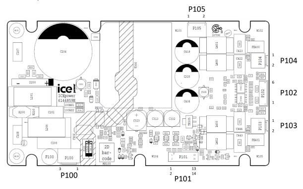
Figure 2: ICEpower100AS1/2 connector overview
