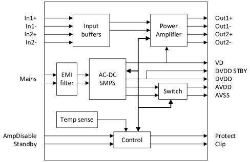
Figure 1: ICEpower100AS1/2 block diagram
