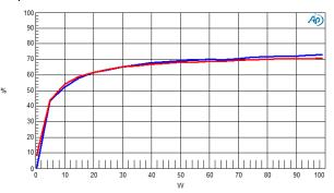
Figure 15: Power efficiency vs. output power per channel, 230V/50Hz (blue), 115V/60Hz (red)
