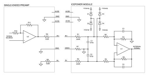
Figure 24: Analog input interface schematics
