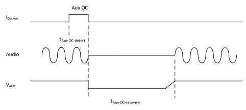
Figure 22: Auxiliary supply overcurrent timing
