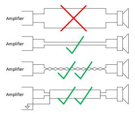
Figure 28: Speaker wire routing
