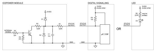
Figure 26: Status output interface schematics
