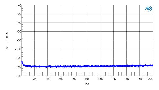
Figure 7: Idle noise (16kFFT) 0-20kHz @ 0dB = 100 W/4  $\Omega$
